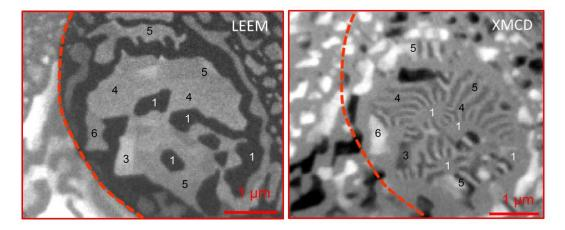
Figure 1. LEEM and XMCD-PEEM images of ultrathin Co/Re(0001) partially covered with carbon. The circular region covered by carbidic and graphitic species is traced by the red dashed line. The Co thickness in atomic layers is marked on the images. The XMCD image is acquired at the Co L-edge, and it shows the magnetic stripe domains typical of out-of-plane magnetization within the carbon-covered region.
